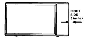
4. Do not install the microwave oven so that the right side is flush with a wall, shelf or cabinet. Leave clearance of at least 5 in. (12.7 cm) on the right side for proper operation. No clearance is required for the left side or top.
