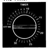
The timer can be set for up to 30 minutes. This controls how long the microwave oven cooks.
