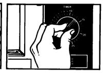
Set the cooking time by turning the Timer Knob clockwise. To reduce the cooking time, turn the Timer Knob counterclockwise.
