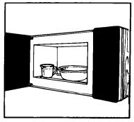
To test a dish for safe use, put it into the oven with a cup of water beside it. Cook on high Cook Power for one minute. If the dish gets hot and water stays cool, do not use it.
