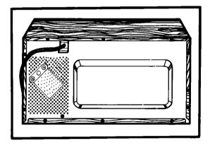
Do not block the rear air intake opening. Blocking the air intake opening can cause damage to the oven and poor cooking results. Make sure the microwave oven legs are in place to ensure proper air flow.
