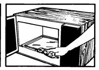
Be sure to clean the surfaces where the door and oven frame touch when closed. When cleaning surfaces, use only mild, non-abrasive soaps or detergents applied with a sponge or soft cloth. Rinse well.
