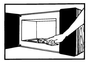
Empty the microwave oven and clean inside it with a soft, damp cloth. Check for damage such as misaligned door, damage around the door or dents inside the oven or on the exterior. If there is any damage, do not operate the unit until it has been checked by an authorized Whirlpool<sup>sM</sup> service technician and any repairs made.
